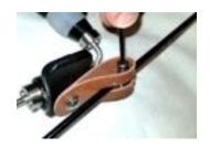
Use a **5/64" Hex Key** to loosen the CROSSBAR clamp screw for adjusting or positioning the control cable housing.
