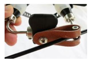
**Step 3**: Loosen setscrew to leave cross-hole clear for cable housing to pass through. Insert CROSSBAR into strap and feed cable housing through cross-hole in CROSSBAR.
