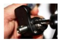
Use a 3/32" Hex Key (Small HSC) or 7/64" Hex Key (Medium & Large HSC) to separate the HSC back halves to change the control cable housing anchor configuration.
