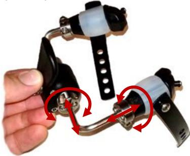
Adjustments shown enable the HSC to accommodate a wide range of anterior-posterior (A-P) and medial-lateral (M-L) anatomical landmark configurations and contact angles. Bicep strap is not shown.
