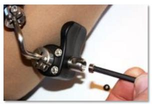
**Step 2:** Remove the jam nut and compression washer from the SWIVEL on the back of the HSC and set aside. Use caution to avoid losing small parts.
