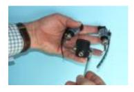
Use a **9/64**" **Hex Key** to loosen or tighten the shaft clamps when adjusting the humeral suspension cuff (HSC) for fitting.
