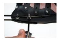
Use a **5/32" Hex Key** to loosen the SWIVEL clamp screw when adjusting or positioning the control cable housing.
