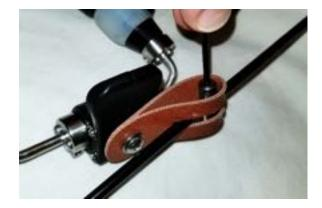
**Step 4**: Tighten setscrew to secure cable housing in CROSSBAR. Use caution to avoid overtightening and thereby crushing the housing or impeding free control cable motion.
