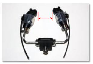
**Step 3:** Slip the HSC onto the user's arm above the elbow from the side. Ensure the space between the contacts is wide enough to pass over the upper arm from the side.
