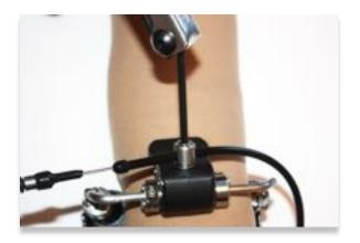
**Step 6:** Gently tighten the jam nut to lock the control cable position in the cable SWIVEL. Large torque is not necessary to lock the cable in position. Use caution to avoid overtightening and thereby crushing the housing or impeding free control cable motion.
