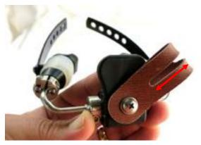
**Step 2**: Verify CROSSBAR strap pivots freely about the pivot post and that longer portion of strap slot faces outward.
